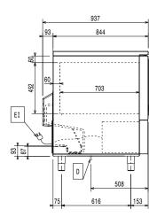
Drain Electrical inlet (power) ΕI Refrigerant Outlet
